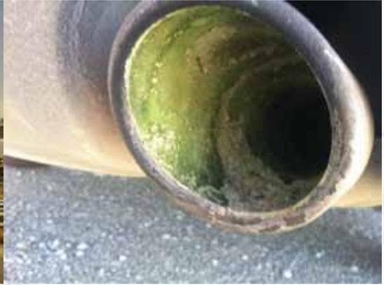
Audi exhaust pipe, after 3000 km of using Iran Diesel fuel – good cetane number, the engine works flawlessly, but the sulphur seems to be in high quantity, at a certain moment the exhaust pipe deposits started to burn and emanate smoke like some smoke candles attached to the car.
